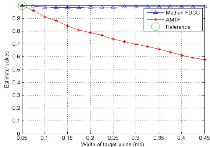
**Figure 2:** FDCC and AMTF parameter values as a function of the pulse width of the second pulse, P2.
